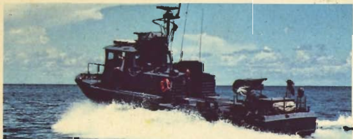
(Above) A Vietnamese "Swift Boat" carries out a Market Time patrol along the coast. This is a PCF Mark II which had a different superstructure from the original variant, in addition, the MARK II was also slightly longer. The armament is covered with canvas to protect it from salt spray. (US Navy)
